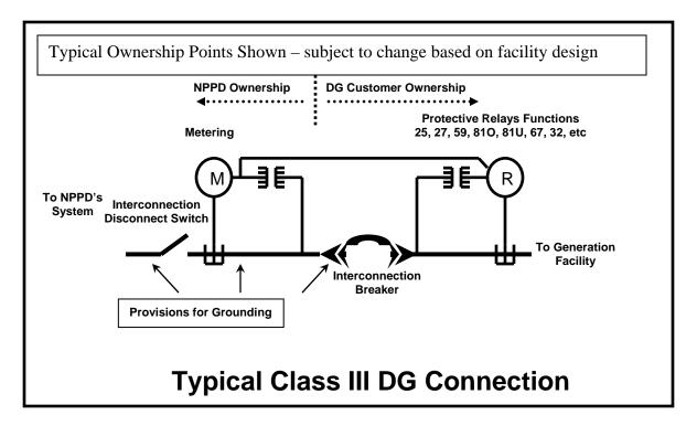
Interconnection protective equipment owned by the DG facility should be maintained and inspected by the DG facility Owner according to the equipment manufacturer's recommendations and/or industry standards. Procedures should be established for visual and operational inspections and for equipment maintenance and testing. Equipment maintained and inspected should include, but not be limited to:
